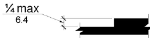
Figure 303.2 Vertical Change in Level
