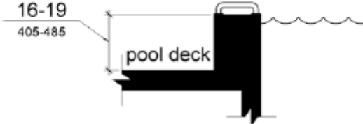
Figure 1009.4.2 Transfer Wall Height
